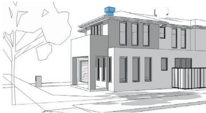
X Non compliant air conditioning unit located at side of roof and above roof ridge line
