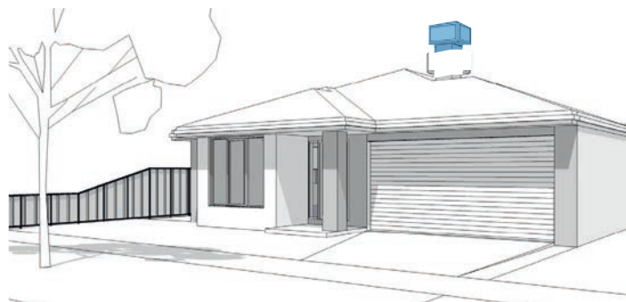
X Non compliant air conditioning unit located at front of roof and above roof ridge line
